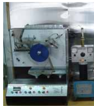
Fig. 1. The assembly Corona electrostatic separator-high voltage source
