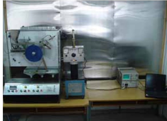
Fig.3. Test setup for measuring conducted emissions
