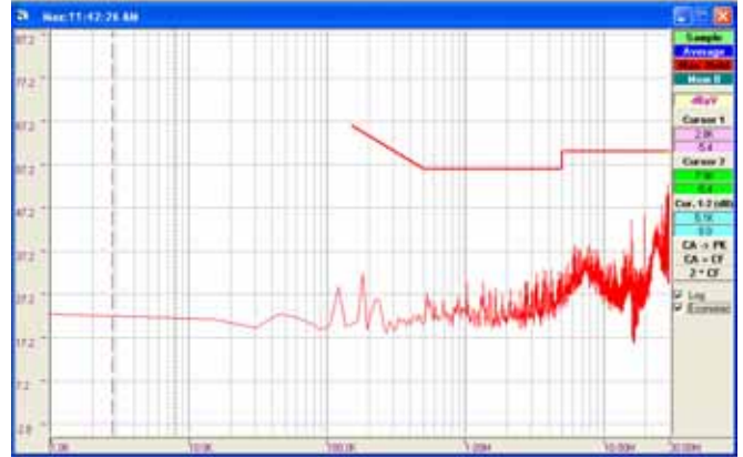
Fig. 14. Diagram of conducted emissions, in Max Hold regime, with the additional filter connected, in logarithmic scale
