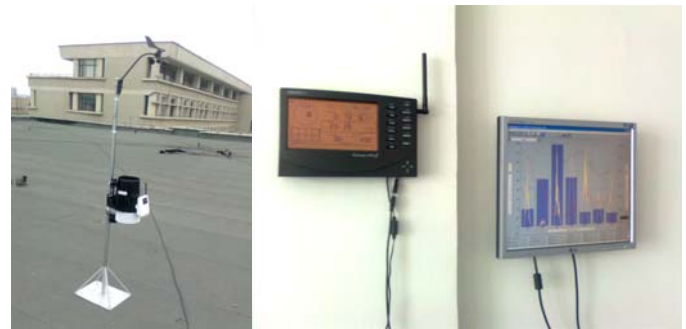
Fig. 3. The Integrated Sensor Suite and the Console modules of the Vantage Pro2™ weather station
