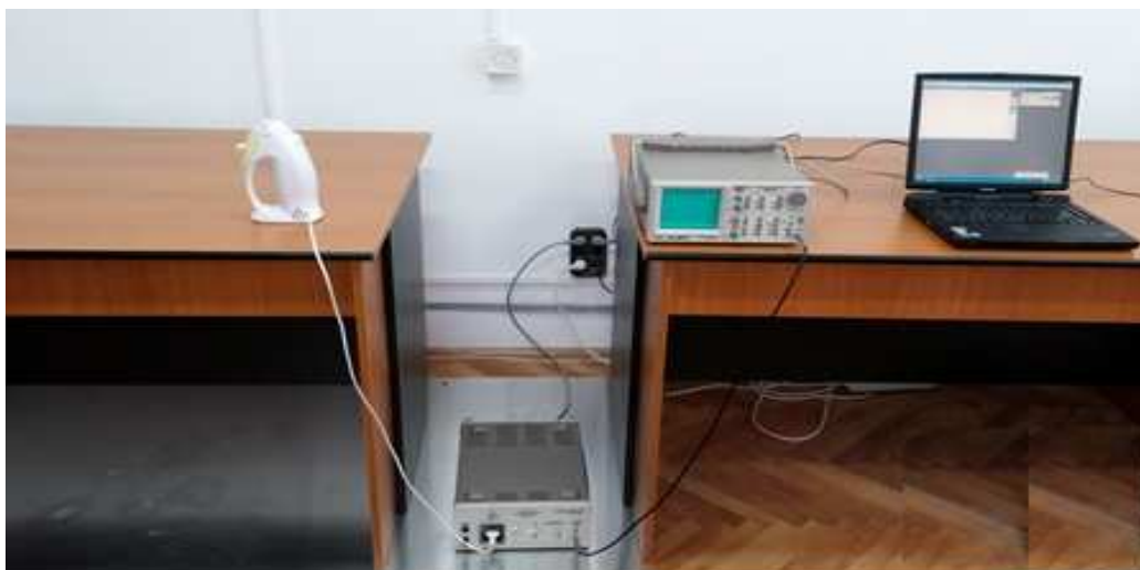
Fig. 3. Test setup for the measurement of the electromagnetic perturbation produced through conduction constructed in the Electromagnetic Compatibility Laboratory from the Technical University of Cluj-Napoca.
