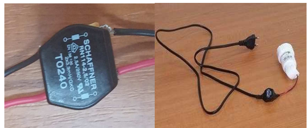
Fig. 12. EMI filter placed in the test setup and its connection.
