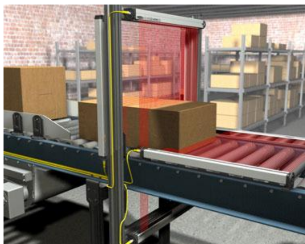
Fig. 11. Tri-dimensional measurement of carton boxes [11].
