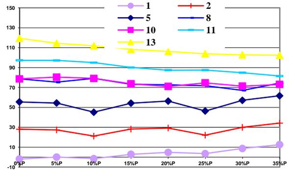
Fig. 7. The reactive power generation when wind farm connected to bus 10.
