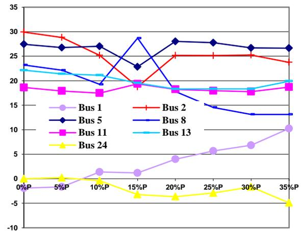
Fig. 8. The reactive power generation when wind farm connected to bus 24.
