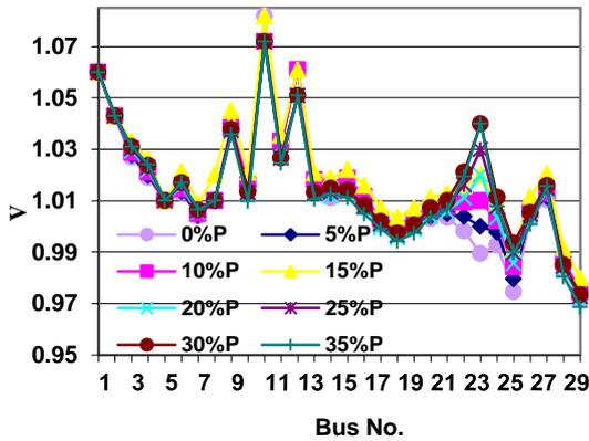
Fig. 4. Voltage profile when wind farm connected to bus 24.
