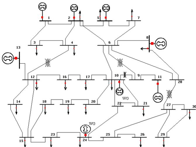
Fig. 1. IEEE 30-bus Electrical system with two Wind generator in bus 10 & bus 24.
