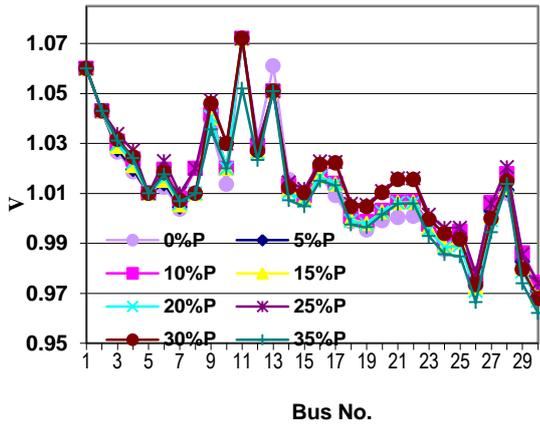
Fig. 3. Voltage profile when wind farm connected to bus 10.
