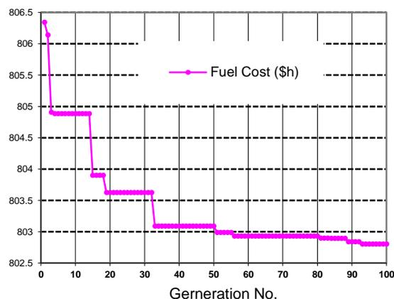
Fig. 2. Convergence characteristics of cost objective function by ED method.
