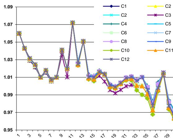
**Fig. 10.** Voltage profile for multiple dispersion on bus 10 and bus 24 with DG 10 High DG 24 Low (%).
