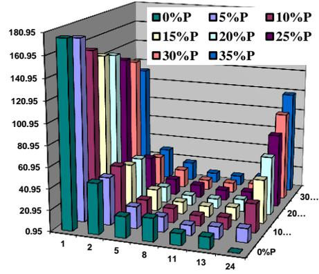
Fig. 6. The active power generation when wind farm connected to bus 24.
