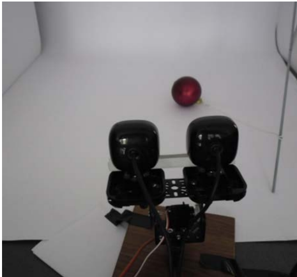
Fig. 10. Tracking the object by the pan/tilt camera system
