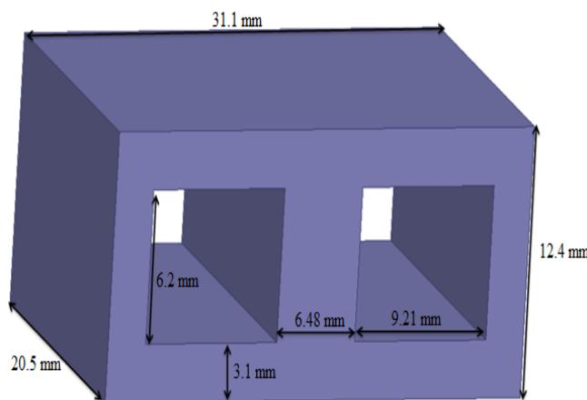
d) Initial geometry for the ferrite core
