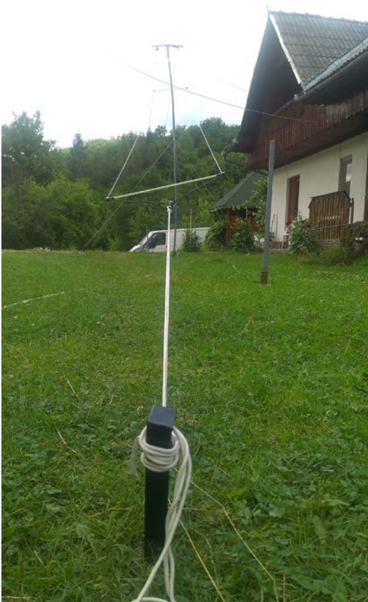
Fig. 3 – Receiving wideband antenna Diamond W330 installed at Lupsa site
