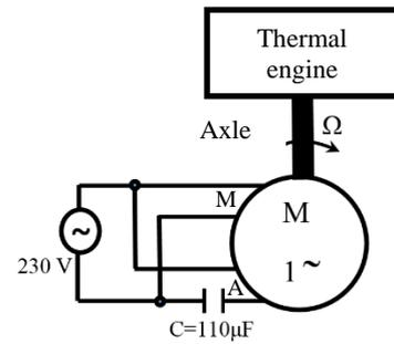
Fig. 2 - Classic connection to the grid of induction machine when used as motor and converted directly to generator.
