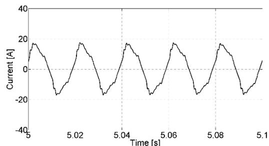
Fig. 11 – Current in the main winding, connected to the power grid.
