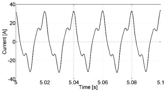
Fig. 6 – Current in the main winding, connected to the power grid.
