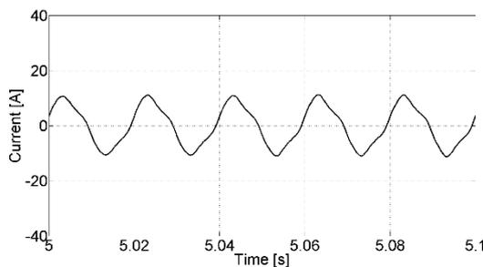
Fig. 16 – Current in the main winding, connected to the power grid.
