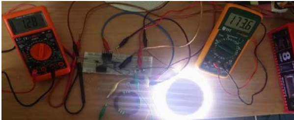
Fig. 13 The current value from the receiver, for the case in which the transmitter is powered with 12V and 80Ah
