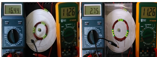
Fig. 9 The value of the voltage induced in the receiver for the case in which the spiral inductors are superimposed and is at 4.3 cm
