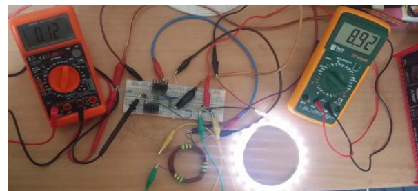
Fig. 16 Current value in the receiver for powering the transmitter with 12V and 80 Ah
