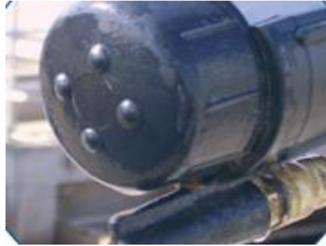
Figure 7 The sensor surface free of any contamination, compressed air cleaning system is not used
