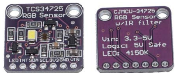
Fig. 3. TCS34725 sensor module with 4150K color temperature LED light Adafruit industries [11].
