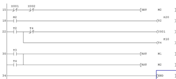
Fig. 5 Ladder diagram for sorting large size objects
