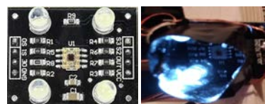
Fig. 7 TCS230 Color sensor and its mounting scheme
