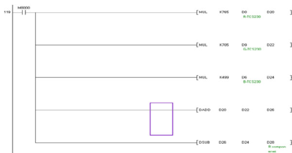
Fig. 11 Ladder diagram for computing the red (R) component
